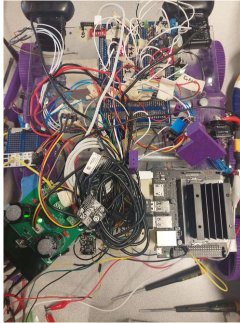
Figure 7. Example of Wire Organization Issues
